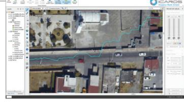
Facilities to divide large projects into tiles/ sheets and combine multiple projects together to produce large orthomosaics, well into the tens of thousands of images, which can be color and tone balanced (Continued)
