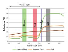
The health of plants can be identified according to how they reflect light in the different wavelengths
